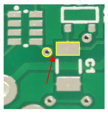
The red arrow is pointing at where the missing path should be. The yellow rectangle and the yellow circle should be connected. It does not matter if this is done before of after C1 has been soldered, but it's probably easier to do it before C1 is populated.
