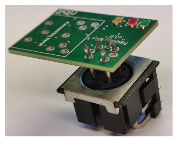
When the pins are soldered you can solder the three LED (with colored lens) in place. The marking in the corner of the colored lens should point to the long side of the circuit board (the one near the top in the image above).
